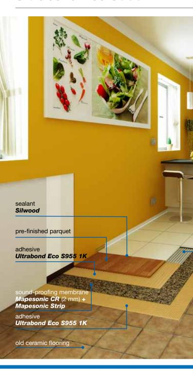
Eco-sustainable system for the rapid installation on existing flooring with under-floor sound-proofing system
