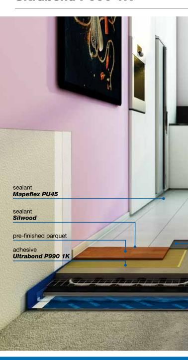
Eco-sustainable system for installing ceramic and pre-finished parquet on heated screeds and on soundproofing systems to reduce the noise of footsteps
