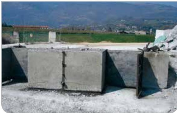
Returned concrete has a high environmental impact on concrete plants and leads to extra operating costs.
