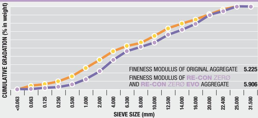
**RE-CON ZERO** and **RE-CON ZERO EVO** aggregates meet the requirements of EN 12620:2008 "Aggregates for concrete".
