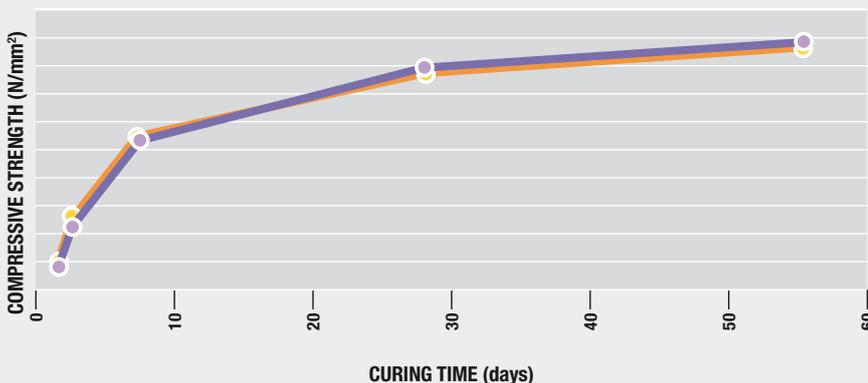
**RE-CON ZERO** and **RE-CON ZERO EVO** aggregates may be used to partially substitute coarse aggregates (up to 50%) in the production of concrete.
