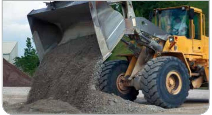
After mixing for a few minutes with **RE-CON ZERO** or **RE-CON ZERO EVO**, concrete is transformed into granular material which may be discharged on the ground and, once cured, used as aggregate in concrete. **RE-CON ZERO** or **RE-CON ZERO EVO** work with all types of concrete.
