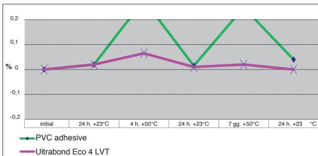
Results of dimensional stability tests carried out on an LVT strip according to EN 1903 standards with **Ultrabond Eco 4 LVT** compared with a generic adhesive for PVC.
