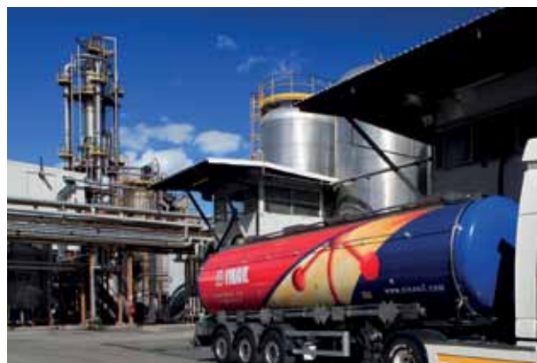
FIG. 4. Loading the product and, in the background on the left, the tubular reactor used for the high pressure copolymerisation of vinylacetate with ethylene at a Vinavil plant.
