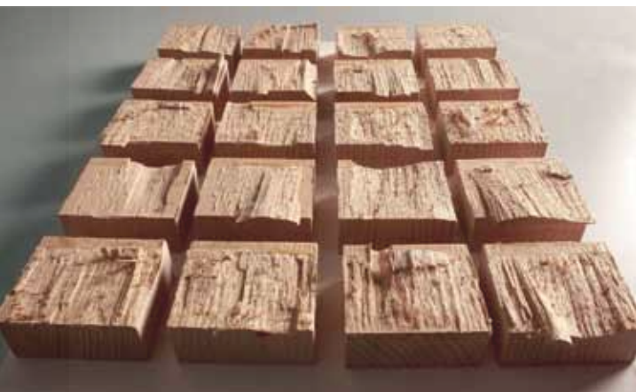
FIG. 3. Assessing the amount of damage to the wood near the joint.
