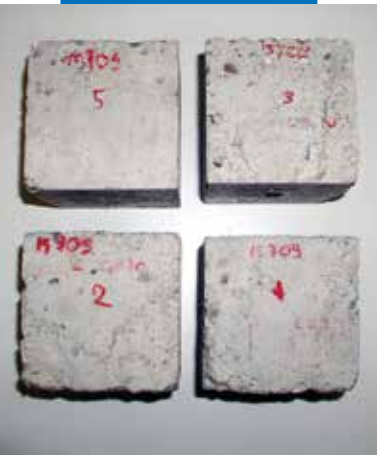
Samples treated with Planiseal WR 90 Gel after freeze-thaw cycles' resistance test
