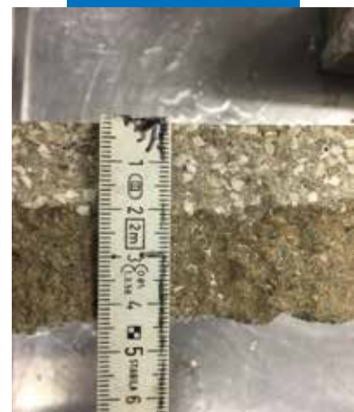
Penetration depth of Planiseal WR 90 Gel
