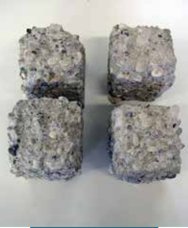
Loss in mass after freeze-thaw cycles' resistance test in samples without the treatment
