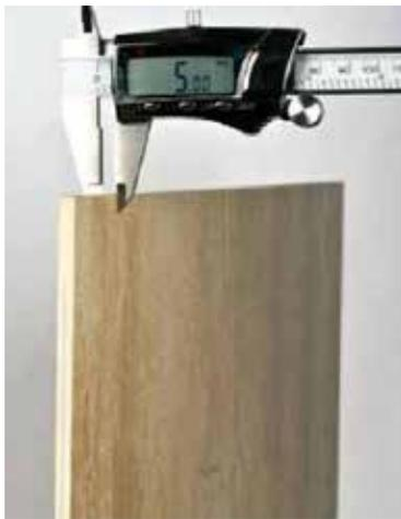
Example of a gauged, 5-mm gauged porcelain tile panel/slab
