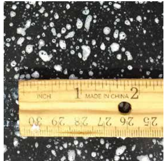
Figure 1: Proper adhesive coverage for vinyl tile and plank
