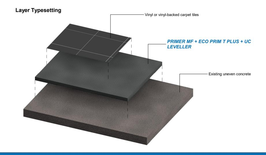
SYSTEM FOR THE INSTALLATION OF CARPET TILES ON UNEVEN CONCRETE WITH HIGH **RESIDUAL MOISTURE CONTENT**
