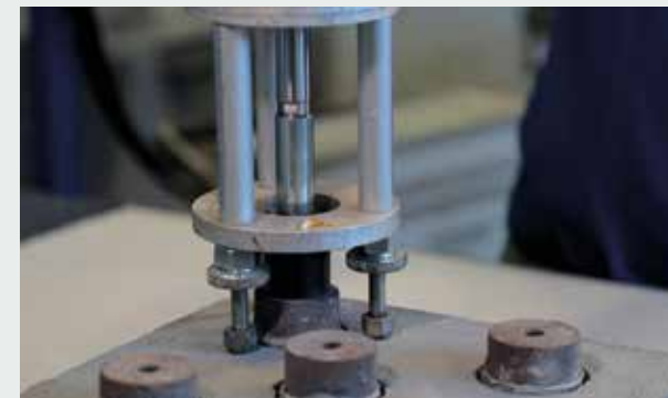
Measurement of bond strength by pull-off according to EN 1542.
