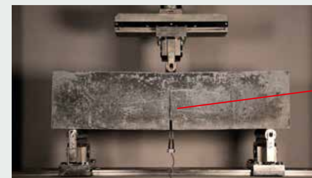
Measurement of residual flexural tensile strength according to EN 14651.
