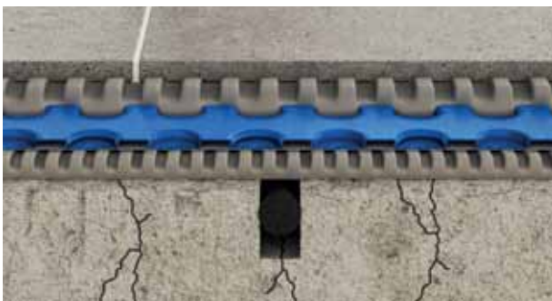
MAPEGUARD UM 35 is an uncoupling, anti-fracture and waterproofing membrane that can be applied on a cementitious screed, without having to copy the layout of control joints in the substrate.
